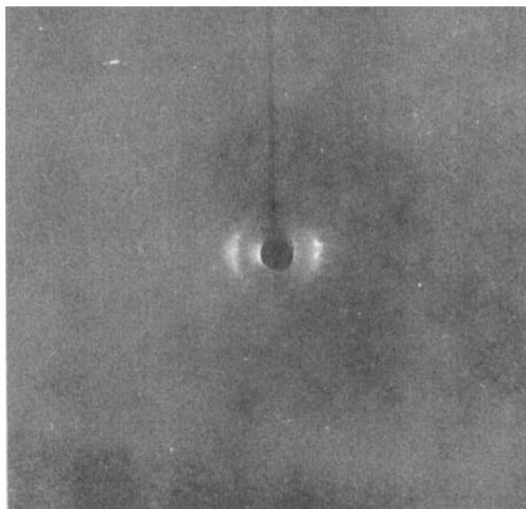
FIGURE 4 X-ray diffraction result with sample LK in 0.7 mm thick capillary (placed in vertical direction in the plane of the figure). Laue camera (Cu Ni filtered radiation), temperature of 55°C. Coexistence of hexagonal ( H_\alpha ) and nematic (N) phases.
